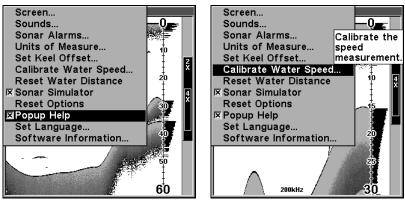
Main Menu (left) with Pop-up Help command highlighted. This example (right) shows the Pop-up Help message for the Calibrate Water Speed command, located on the Main Menu.
